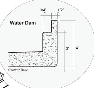
Water dam is omitted at threshold side of the base when using the independent barrier-free threshold
