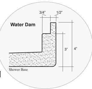
Water dam is omitted at threshold side of the base when using the integral accessible threshold
