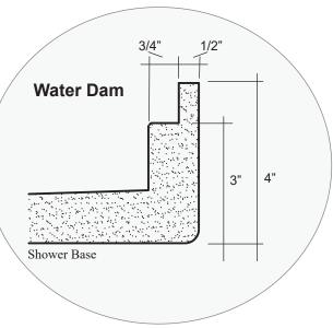
Water dam is provided on all sides of the base when using the raised threshold
